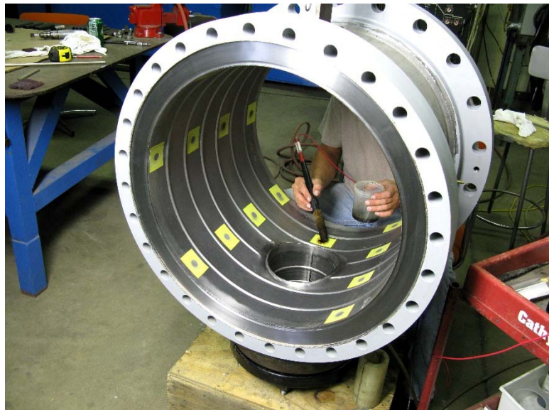
Figure 1 Platinum spots being electroplated onto a tantalum-lined heat exchanger bonnet in Tricor's shop.
